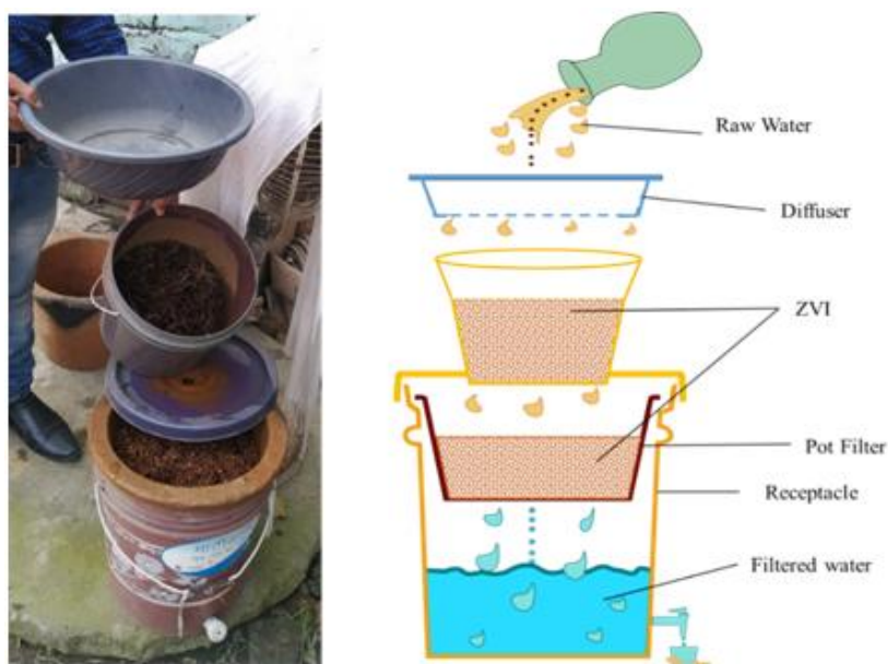
Figure 4: Integration of two-stage ZVI into MatiKalp with diffuser
